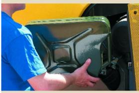
Easy fuel filling, even directly form a fuel can without spout of funnel.
