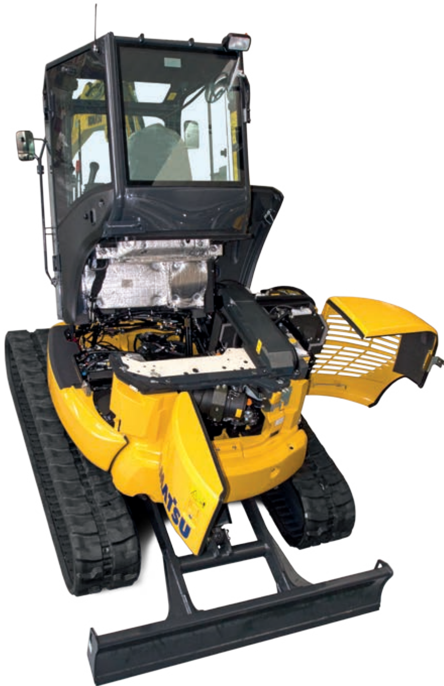
Rear bonnets for quick engine checks, simple inspections, cleaning of the radiators and easy access to the battery
